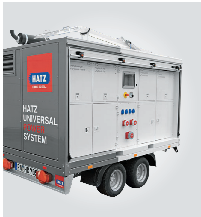
The Hatz HUPS concept study (Hatz Universal Power System) as a trailer-mounted design. The mobile system includes a 150-bar, high-pressure cleaner, two hydraulic pressure modules delivering 200 or 700 bar, an electricity supply up to 63 A and a 15-bar compressed air compressor. A LED light tower mast is mounted on the roof. The basic energy is supplied by a Hatz 3L41C 25 kW diesel engine and a 25 kVA generator. The system can be operated using a touchscreen display or using the UMTS/GPS module and remote control.
