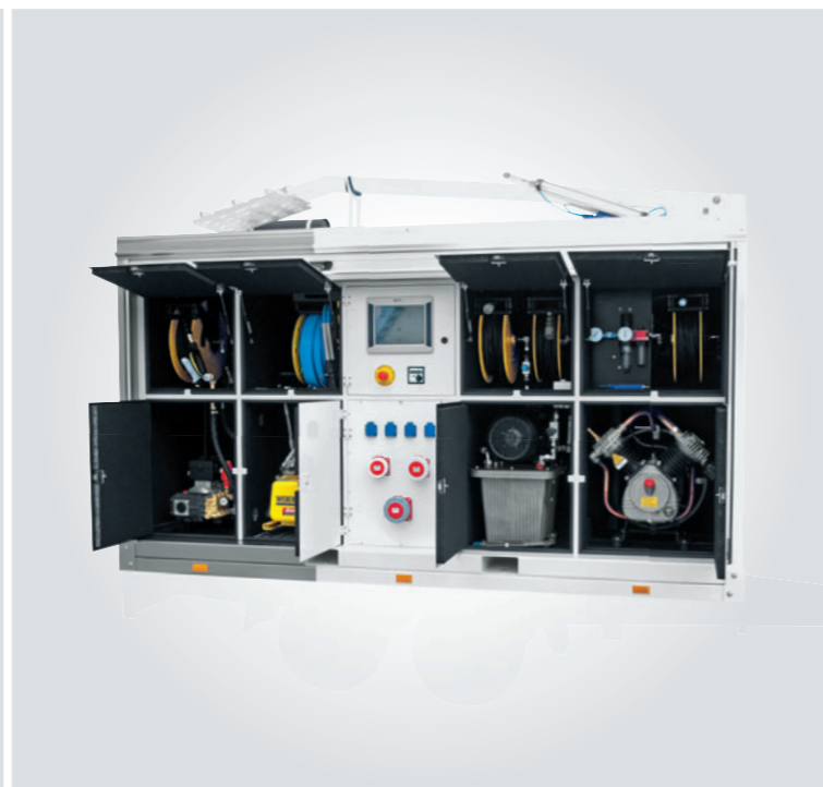
The Hatz HUPS concept study (Hatz Universal Power System) as a trailer-mounted design. The mobile system includes a 150-bar, high-pressure cleaner, two hydraulic pressure modules delivering 200 or 700 bar, an electricity supply up to 63 A and a 15-bar compressed air compressor. A LED light tower mast is mounted on the roof. The basic energy is supplied by a Hatz 3L41C 25 kW diesel engine and a 25 kVA generator. The system can be operated using a touchscreen display or using the UMTS/GPS module and remote control.
